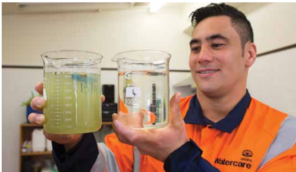
Spot the difference: Plant operator Abe Tahere holds samples of raw wastewater that enters our treatment plants (left) and the treated wastewater that is ready to be discharged (right).
